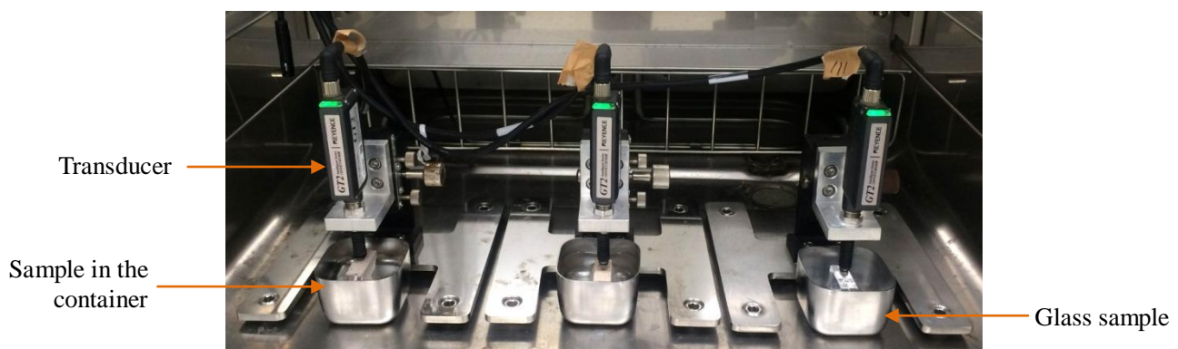
Photo 1 Experimental setup with specimen in the first two container(from left), the third container has a glass to account for thermal expansion of transducers.
